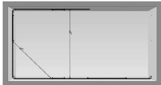
The profile elements of the central part of the ceiling structure are pushed as far as possible in the first part after it is installed.
